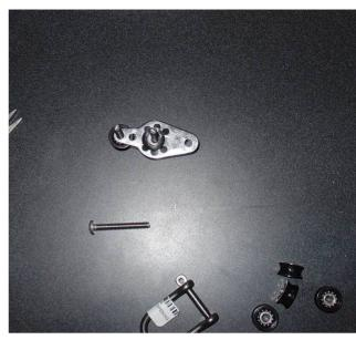
add cheeks and sheaves (and 1 becket on small sheave side with appropriate washers on large block side)
