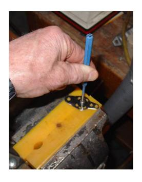
Drive the axle through the bushing and bottom cheek. Flatten the flares on both sides
