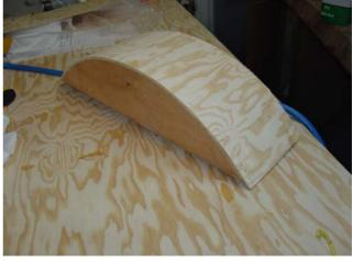
Cut two pieces of ¼ plywood 10" wide and 30" long across the grain of the plywood as shown. Staple or nail one piece of plywood on the forms allowing it to hand over each form 1" (not as shown—but better)
